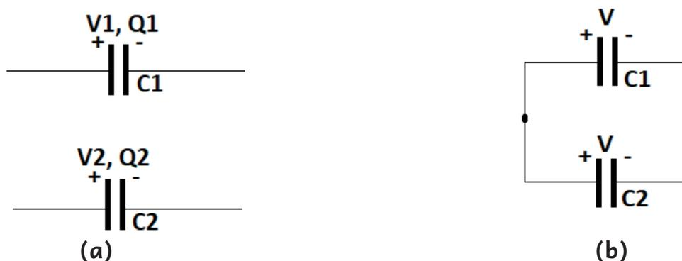
In **Figure (a)**, two capacitors of capacitances  $C_1$  and  $C_2$  are charged to potentials of  $V_1$  and  $V_2$ , respectively with  $V_1 > V_2$ .
